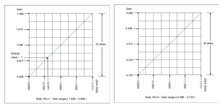
The 6 bits (bit 5~bit 0) of the configuration register set the gain of output current, i.e., G. As total 6-bit in number, i.e., ranged from 6φ000000 to 6φ111111, these bits allow the user to set the output current gain up to 64 levels. These bits can be further defined inside configuration register as follows:
