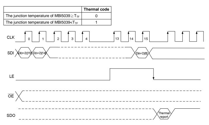
At the falling edge of LE, if the driver is overheated, the code %7FF(HEX)+is delivered to SDO; otherwise, the code %7FFF(HEX)+is latched to sift register.
