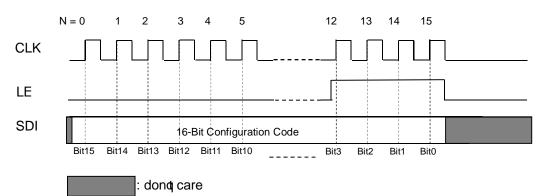
After entering the writing configuration mode, the system controller sends a 16-bit configuration register setting which must include check bits (bit9~bit6 = 0101) to the 16-bit shift register through the SDI pin. Then the falling edge of LE will transfer the contents in the shift register to a 16-bit configuration register rather than the 16-bit output latch. If the check bits are not equal to 00101+, the data will not be updated to the configuration register.
