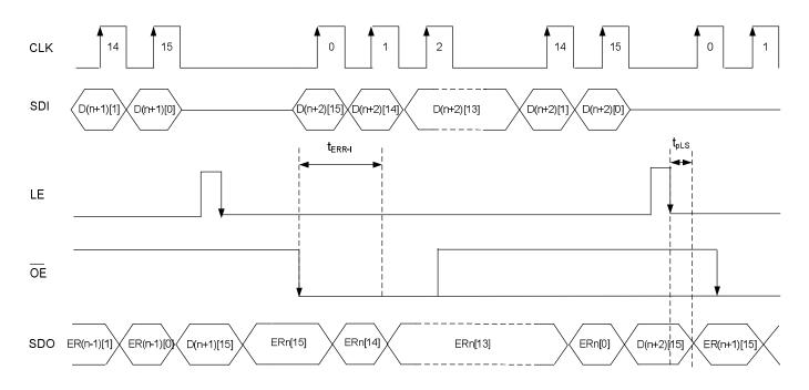
1. Condition of valid error detection: (1) Data =+1+(2)  $\overline{OE}$  (low) > t<sub>ERR-I</sub> Note: If the above condition is not matched, the error detection is suppressed and error codes remain %
