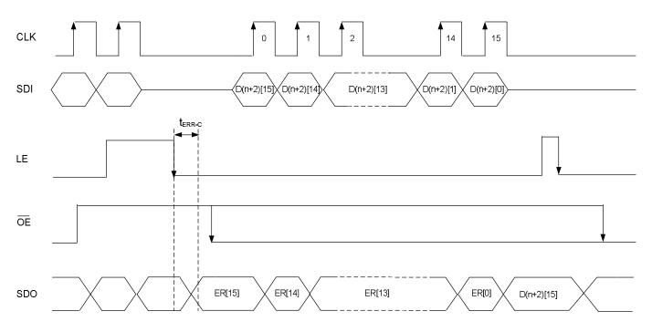
1. Conditions required to activate the open-circuit detection: (1) falling edge of LE and (2)  $\overline{OE}$  =High
