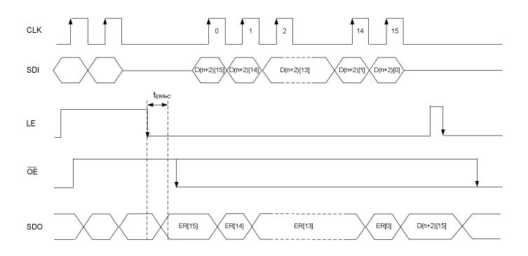
1. Conditions required to activate the short-circuit detection: (1) falling edge of LE and (2)  $\overline{OE}$  =High
