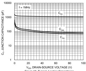
Figure 10. Typical Junction Capacitance
