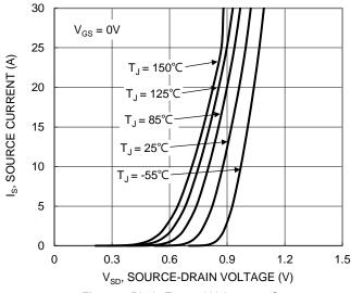
Figure 9. Diode Forward Voltage vs. Current
