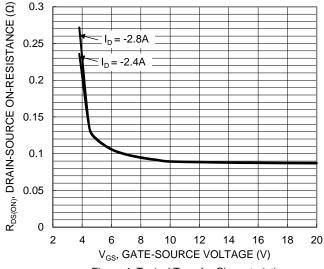
Figure 4. Typical Transfer Characteristic
