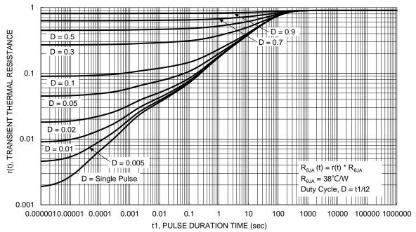
Figure 13. Transient Thermal Resistance
