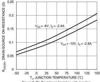
Figure 7. On-Resistance Variation with Junction Temperature
