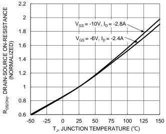
Figure 6. On-Resistance Variation with Junction Temperature
