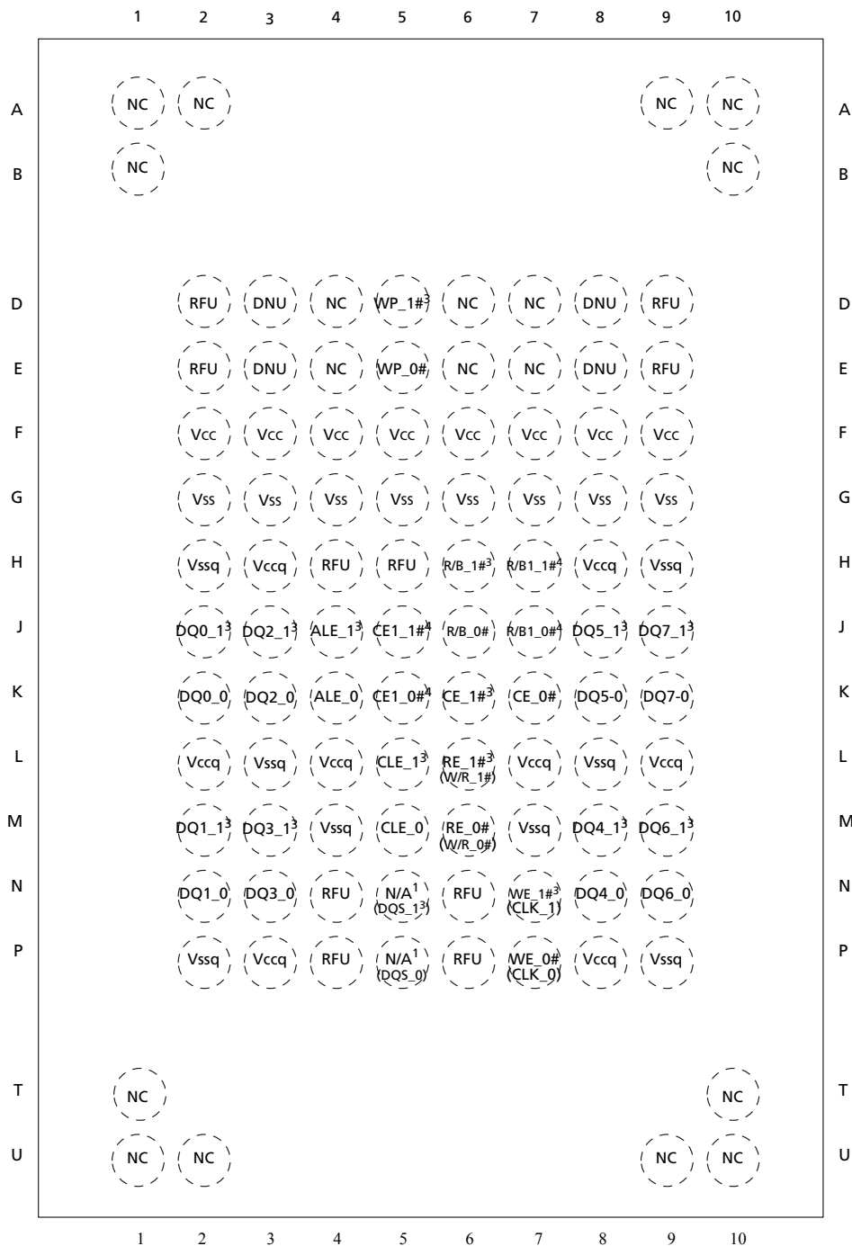
Figure 3: 100-Ball BGA (Ball-Down, Top View)
