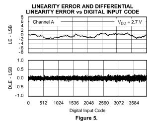
LINEARITY ERROR AND DIFFERENTIAL LINEARITY ERROR vs DIGITAL INPUT CODE
