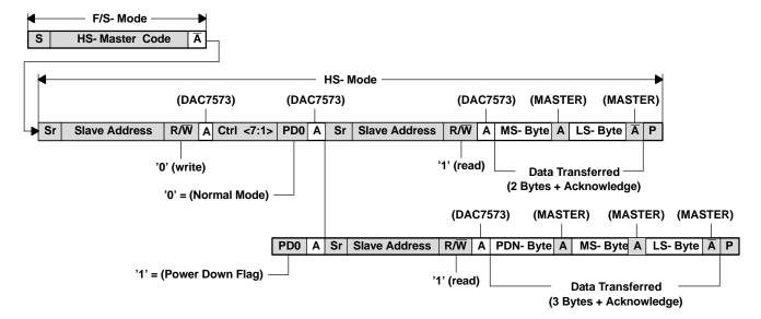
Figure 38. High-Speed Mode: Slave Transmitter
