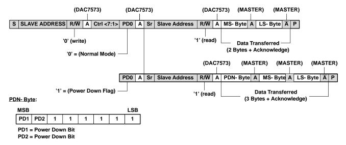
Figure 37. Standard and Fast Mode: Slave Transmitter
