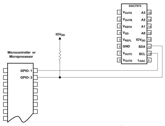
NOTE: DAC7573 power and input/output connections are omitted for clarity, except I<sup>2</sup>C Inputs.
