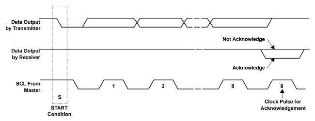
Figure 33. Acknowledge on the I<sup>2</sup>C Bus
