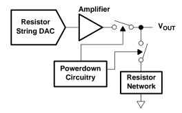
Figure 39. Output Stage During Power Down
