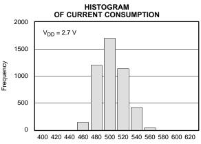
$I_{\mbox{\scriptsize DD}}$  - Current Consumption -  $\mbox{\scriptsize $\mu$A}$ Figure 21.
