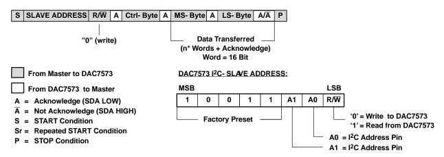
Figure 35. Standard and Fast Mode: Slave Receiver
