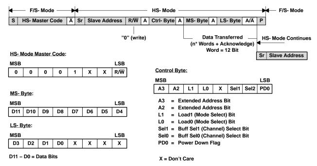
Figure 36. High-Speed Mode: Slave Receiver
